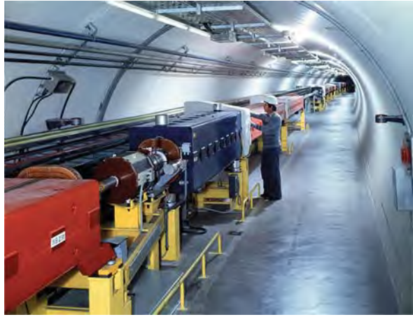
Fig. 3.17 Inside the tunnel housing the Super Proton Synchrotron (SPS) in CERN. The blue blocks are quadrupoles and the red blocks are bending magnets. All magnets are conventional ferromagnets. Photograph copyright CERN
