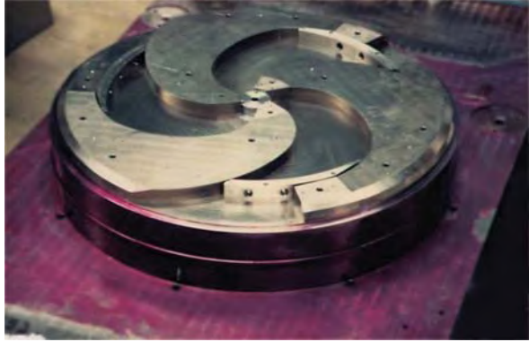
Fig. 3.10 Pole pieces of the GANIL injector cyclotron. The hills and valleys creating the azimuthally varying fields are given a spiralling shape to further enhance the focusing effect. Photograph by courtesy of Eric Baron [11]
