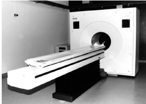
Fig. 6.31 The Siemens ECAT EXACT HR clinical PET scanner. It contains 25'088 LSO crystals measuring 5.9 \times 2.9 \times 30 \text{ mm}^2 and arranged in a 15 cm long cylinder surrounding the patient. This ring of detectors is hidden in the square box shown behind the patient's bed. Photography courtesy of Siemens
