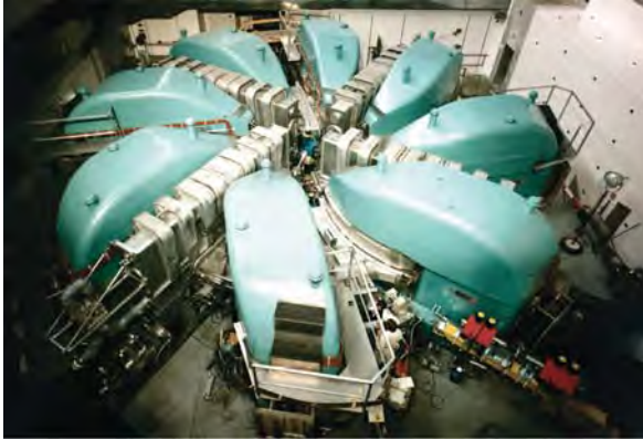
Fig. 3.12 One of the most powerful cyclotrons in the world today is at the Paul Scherrer Institute in Switzerland near Zurich. The PSI 590 MeV ring cyclotron for high-intensity proton beams started its operation in 1974. It is based on a design proposed by Hans Alexander Willax [12] in 1963. Originally designed for 100 microampere, it now produces beam intensities of 2 mA, with a further increase in preparation. The 20-fold increase became possible by replacing the original injector (a one solid pole cyclotron) with a new separate sector cyclotron and by increasing the RF power for acceleration. The main parameters of the machine are given in Table 3.5. Figure by courtesy of the Paul Scherrer Institute, Switzerland
